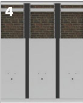
4. Place the cladding panels up to the height of the connections / fixtures and cut openings for the connections / fixtures.
