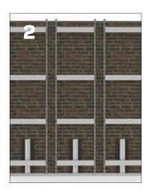
Place the steel frames for cladding on the profile, align, and attach them to the masonry wall.
